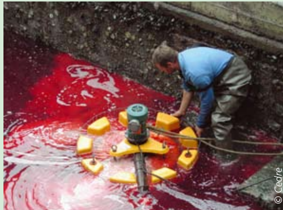
Recommended use of a surface skimmer.
