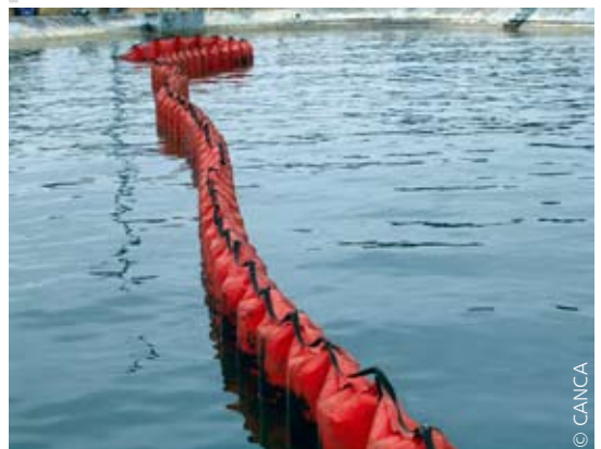
Boom deployed on the water surface.
