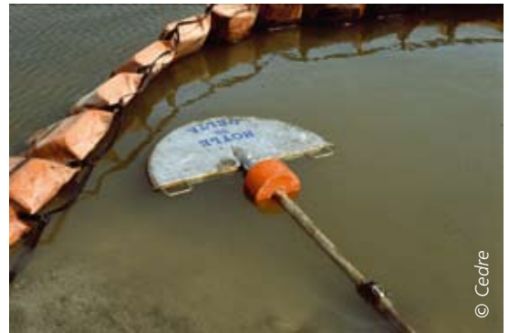
Lightweight flat suction head for floating pollutant.
