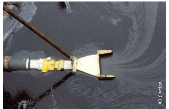
Suction head with a wide opening, equipped with an arm designed to correctly position it on the slick.
