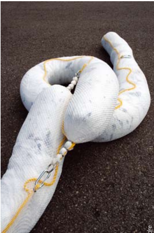
Sorbent boom sections connected with overlap.
