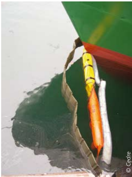
Fence boom (grey), curtain boom with foam-filled floats (orange), self-inflating curtain boom (yellow), sorbent boom (white).
