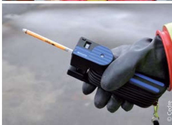
Detection of vapours by photo-ionisation (top) and with an indicator tube (bottom)
